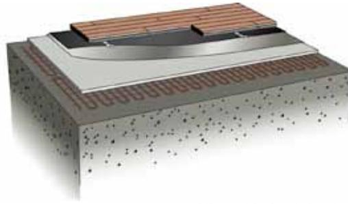
Wood floor with electric heating on existing concrete floor
